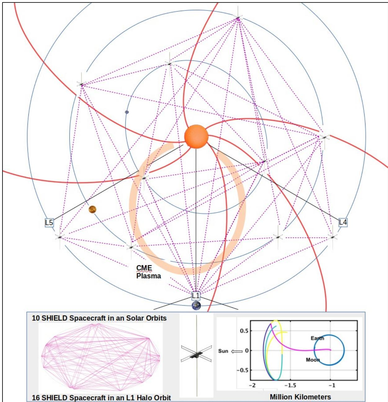
Figure 4. Conceptual depiction of “Big SHIELD,” a notional flagship-class tomographic constellation that images ICME structure and magnetic field before the ICME reaches the Earth’s magnetosphere. Radio paths are magenta, orbits blue, ICME plasma is orange. Not to scale.
