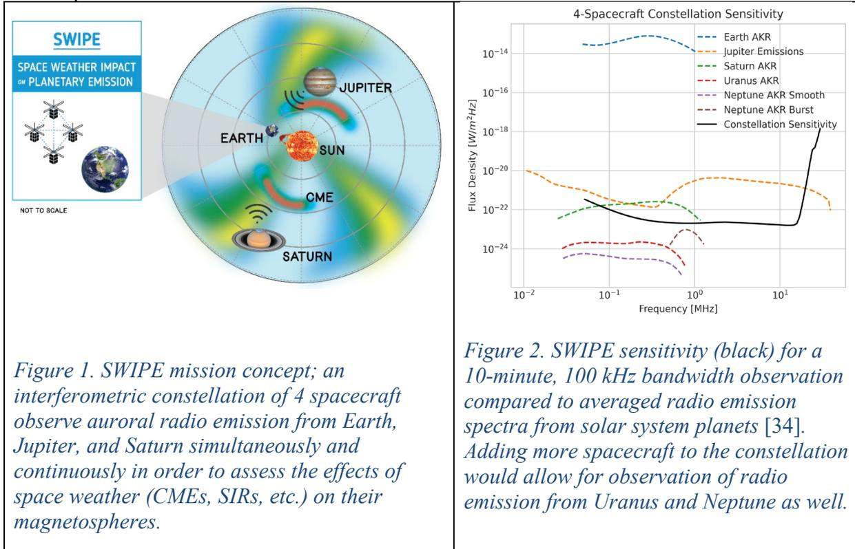
Figure 1. SWIPE mission concept; an interferometric constellation of 4 spacecraft observe auroral radio emission from Earth, Jupiter, and Saturn simultaneously and continuously in order to assess the effects of space weather (CMEs, SIRs, etc.) on their magnetospheres.
