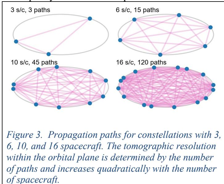
Beacon tomography offers a densely sampled volumetric view of the spatial and temporal structure of ICMEs approaching the Earth. Over sufficiently long propagation paths, this technique could revolutionize space weather forecasting. In beacon tomography mode, SHIELD measures total electron content (TEC) and magnetic field properties on propagation paths between spacecraft.
