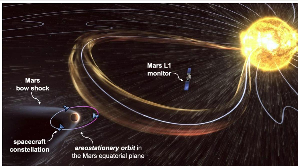
**Figure 3.** Concept of upstream monitors at Mars L1 and in areostationary orbit (the Mars-equivalent of geostationary orbit) situated in the Mars equatorial plane. Image adapted from NASA/GSFC.
