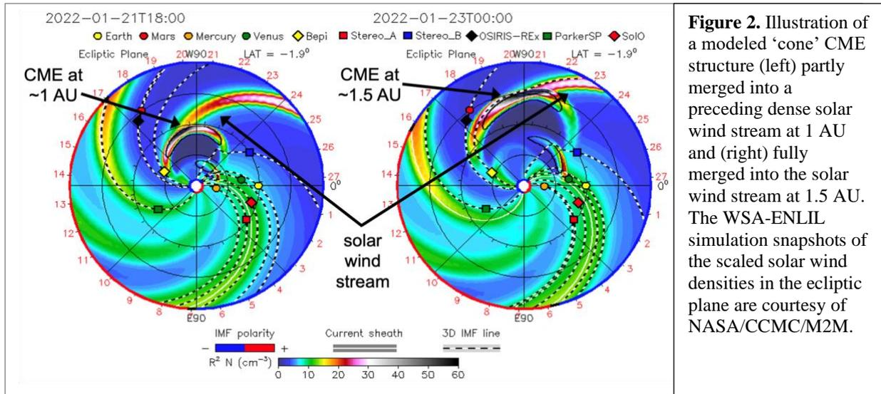
**Figure 2.** Illustration of a modeled ‘cone’ CME structure (left) partly merged into a preceding dense solar wind stream at 1 AU and (right) fully merged into the solar wind stream at 1.5 AU. The WSA-ENLIL simulation snapshots of the scaled solar wind densities in the ecliptic plane are courtesy of NASA/CCMC/M2M.
